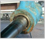
The above photo shows how cleaning the strut face thoroughly will clearly reveal the bearing outer shell for the most accurate measuring.
