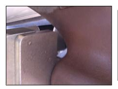
This close up photo shows a wakeboard boat strut with the horseshoe inverted and facing upward. This method provides clearance so the horseshoe does not contact the leading edge of the strut.
