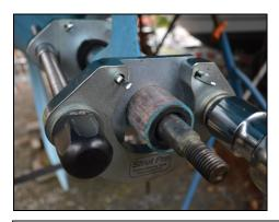
*Tip!* Place your new bearing over the back of the prop shaft and butt it up the old bearing. This now becomes a perfect pilot alignment. Next rest the aft horseshoe on the new bearing. This provides you perfect alignment for the old bearing to slide through the aft horseshoe.
