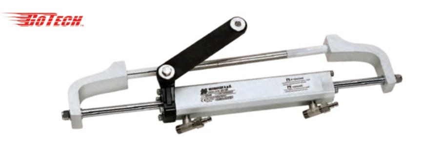
UC81-OBF - Balanced: the number of turns lock-to-lock is equal port to starboard and vice-versa. Front mount cylinder for outboard engines up to 115 hp Replaceable cylinder end caps
